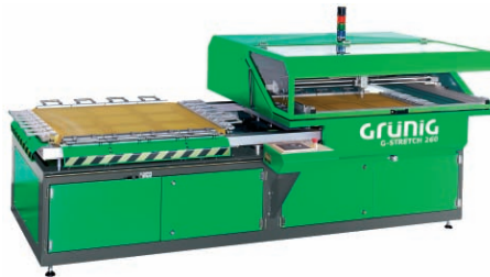
G-STRETCH 260 Double stretching table with robot for glueing
